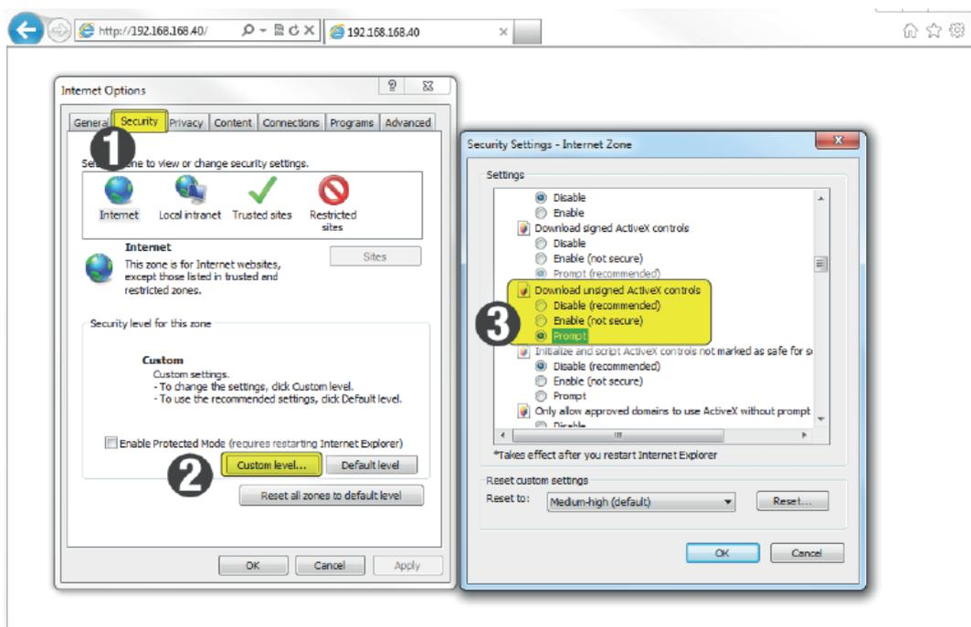
2. Please enter the camera's IP address in the address bar and click on "Enter" (The default IP address is "192.168.1.86" ), then the system will show you the login interface. Then, input your camera's "User Name" (Default: admin), "Password" (Default: 123456) and click on "Login".
